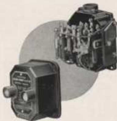
Type "SCI" push-button starter with magnetic over-current relays for control of squirrel-cage motors up to 7½ H.P.
